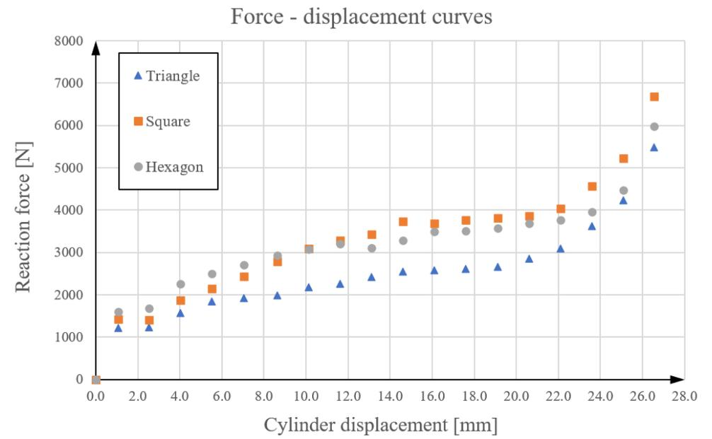
Force - displacement curves for different cell structures
