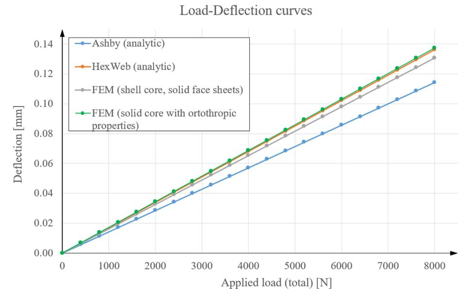
Hexagon cell displacement FEM vs. Analytic
