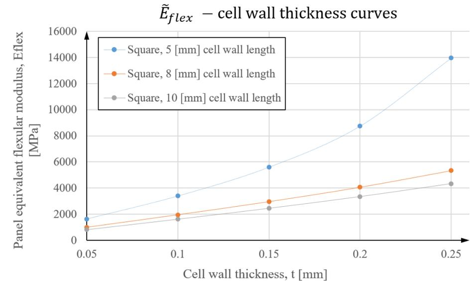
Square cell structure equivalent flexural modulus curves
